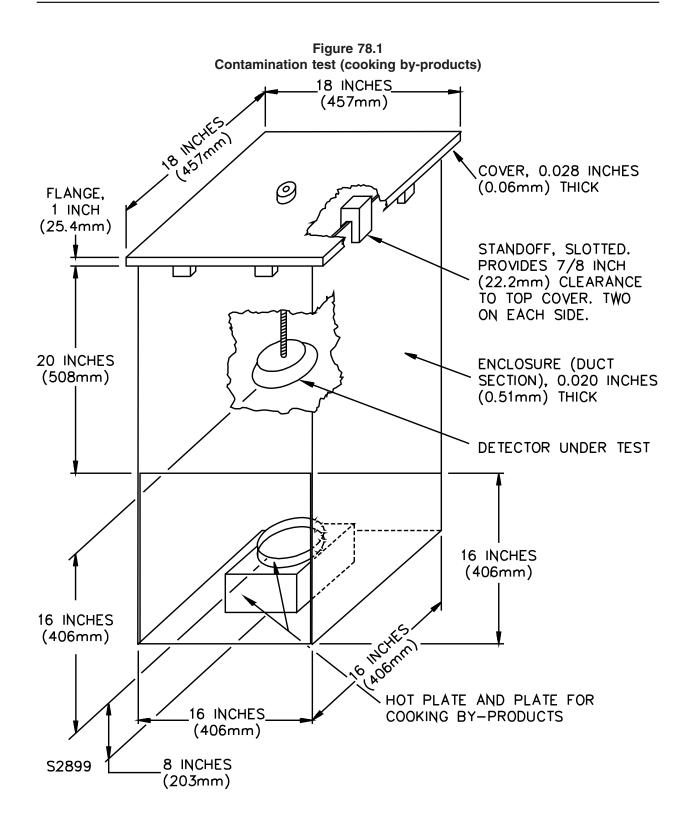
78.4 The alarm under test is to be supported on the end of a threaded 1/4 inch (6.4 mm) steel rod positioned so that the exposed face of the alarm is approximately 12 inches (304 mm) below the enclosure cover and 16 inches (406 mm) above the aluminum plate. The alarm is not to be energized during the test.
