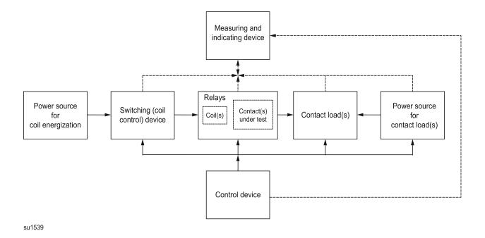
NOTE The relays under test include any suppression and/or indicating device.
