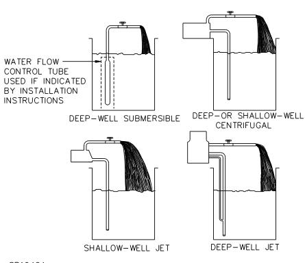
Figure 40.1 Maximum normal load test set-ups
