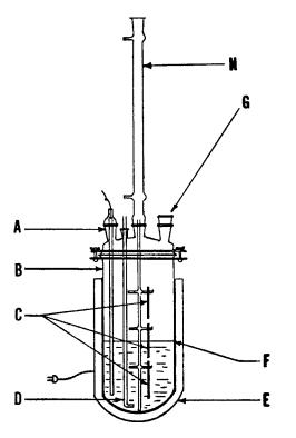
NOTE 1—A = thermometer port, B = flask, C = specimens hung on supporting device, D = air inlet, E = heating mantle, F = liquid interface, G = opening in flask for additional apparatus that may be required, and H = reflux condenser.
