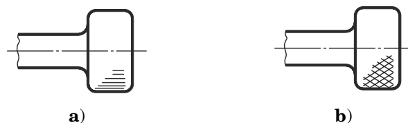
Figure 84 Examples of representation of knurled part
