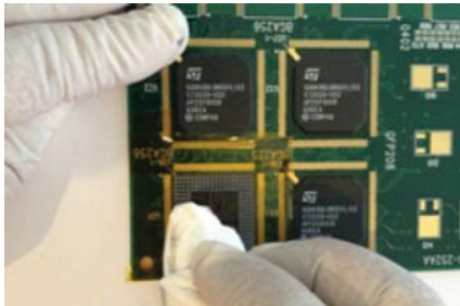
Figure 6 Wipe off excess solder paste
