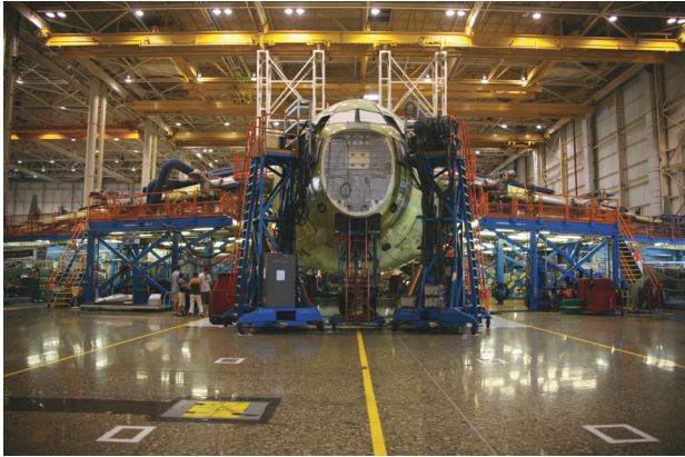
Figure 17-1. Aircraft assembly areas require lighting from multiple sources and multiple angles, including onto the underside of the wings. (©Canstock)
