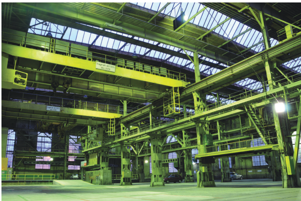
Figure 17-2. Overhead and side windows combined with electric lighting provide relatively uniform lighting in this space. The light colored floor reflects light to the underside of the large structures. (Image from iStock / PatrickHutter)
