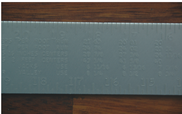
Figure 18-1. Left: Metal ruler illuminated with an ambient lighting system. Right: Same object illuminated with a task light adjusted to reveal the embossed figures. (Images courtesy of Lighting Forensics LLC)
