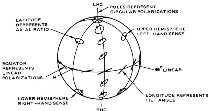
**Figure 46—Representation of Polarization on the Poincaré Sphere**
