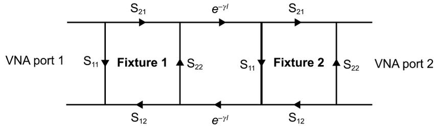
Figure E.6—Line standard signal flow graph
