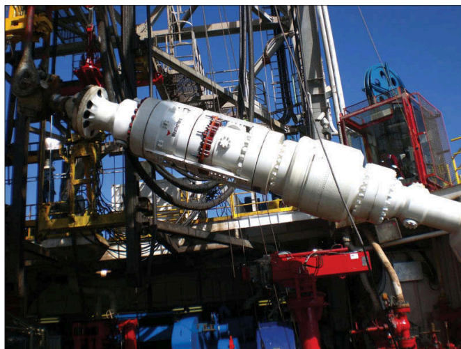
Weatherford's Model 7875 BTR RCD is helping to extend MPD capabilities to deepwater drilling operations from dynamically positioned drilling vessels.
