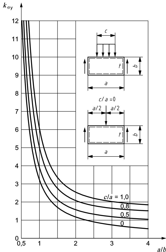
**Figure 11 — Buckling factor  $k_{\sigma y}$**
