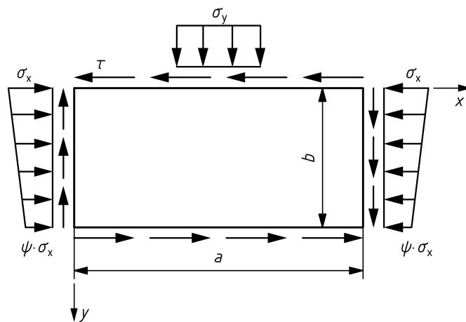
**Figure 10 — Stresses applied to plate field**
