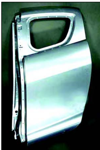
(A) Door Structure Spot-Welded for Impact Stability
