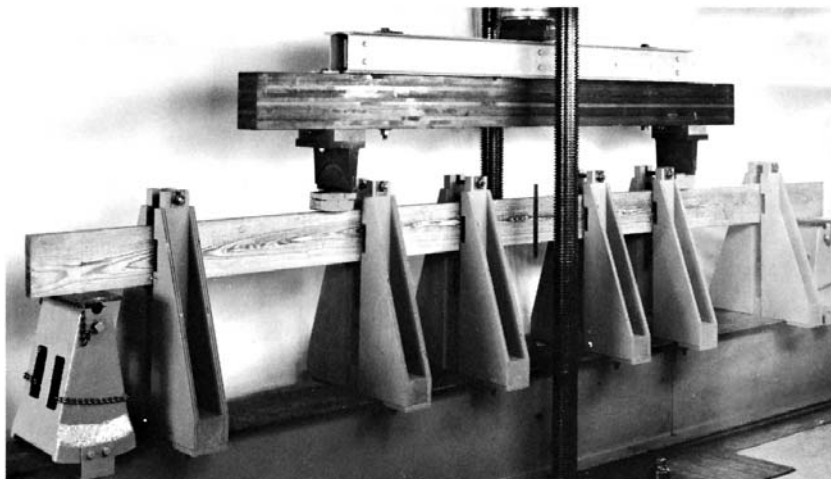
FIG. 3 Example of Lateral Support for Long, Deep Flexure Specimens
