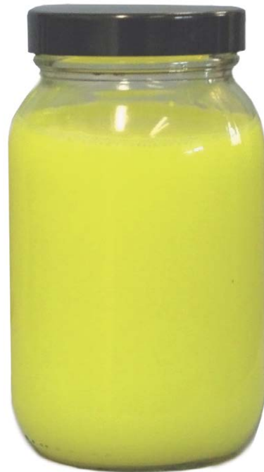
Figure 8. Typical wastewater from fluorescent penetrant test rinse stage.
