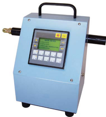
Figure 33. Air flow meter with orifice and differential pressure transducer: (a) photograph; (b) pneumatic circuit.
