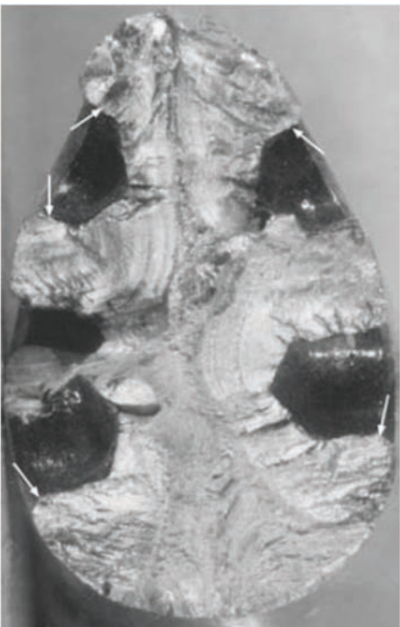
Fig. 25 Multiple fatigue initiations at through-wall drill holes in user-modified bicycle handlebar stem. Original magnification: 3×
