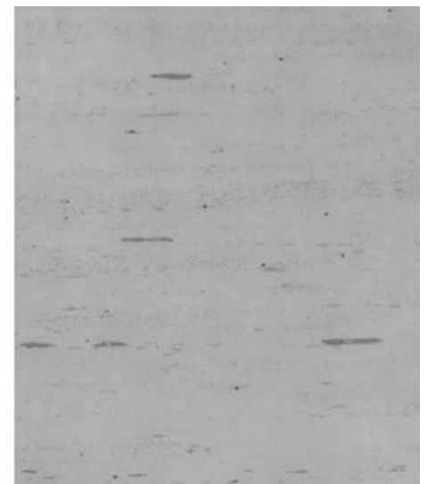
Fig. 13 Significant volume fraction of manganese sulfide inclusions in wedge-shaped tapered ring microstructure. Original magnification: 73×
