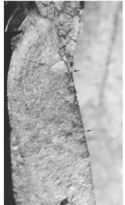
Fig. 22 Compressor blade fracture surface showing fatigue origins on low-pressure (i.e., right) side of blade, as indicated by the arrows. Original magnification: 13×
