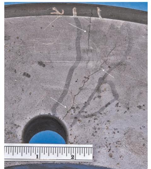
**Fig. 14** Photograph of stress-corrosion cracking (arrows) observed on the outside surface of a steam turbine rotor disk
