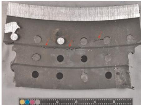
**Fig. 11** View of stress-corrosion cracks (arrows) on the upstream side of a steam turbine disk. Plastic deformation or thinning was not observed adjacent to the stress-corrosion cracks.
