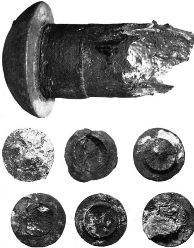
**Fig. 5** Photographs of a cracked rivet (top) and dislodged rivet heads (bottom) from a boiler that experienced caustic stress-corrosion cracking. Source: Ref 5
