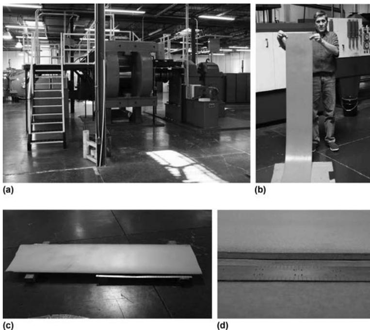
Fig. 6 (a) Direct powder rolling mill, (b) 0.25 mm (0.010 in.) thick porous Ti strip, (c) and (d) 6.35 mm (0.25 in.) thick Ti-6Al-4V direct powder rolled plate. Courtesy ADMA Products, Inc.
