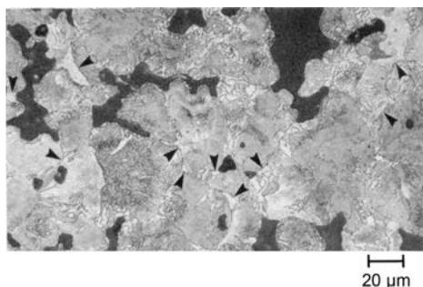
**Fig. 12** Free copper (see arrows) that precipitated from solution in a PM copper steel (FC-0508)
