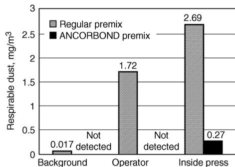
**Fig. 5** Respirable dust in the work area of a plant for manufacturing PM parts Source: Ref 1
