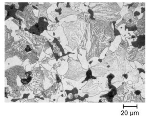
**Fig. 6** Ferrite-pearlite microstructure of an as-sintered PM carbon steel (F-0005)
