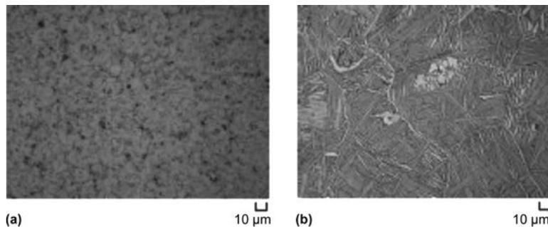
**Fig. 12** The microstructure of thin gage sheet samples of (a) roll compacted titanium and (b) roll compacted Ti-6Al-4V. Source: Ref 16
