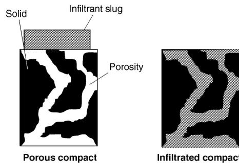
**Fig. 14** Schematic of copper infiltration
