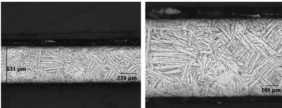
Fig. 7 Microstructures of PM direct powder rolled Ti-6Al-4V strips produced from ADMA titanium powder. UTS = 965 MPa (140 ksi), YS = 848 MPa (123 ksi), El = 12.5%
