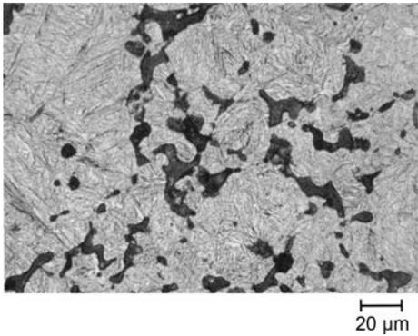
**Fig. 7** Tempered martensitic microstructure of a quench-hardened and tempered PM carbon steel (F-0008)
