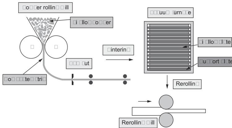
Fig. 5 Schematic of room temperature direct powder rolling. Courtesy ADMA Products, Inc.
