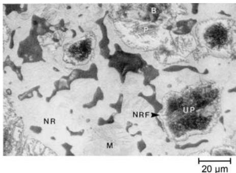
**Fig. 3** As-sintered microstructure of a part made of a diffusion-alloyed powder FD-0405: B, bainite; P, pearlite; UP, unresolved pearlite; NR, nickel-rich region; NRF, nickel-rich ferrite; M, martensite
