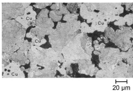
**Fig. 11** Free copper in a PM copper steel (FC-0508) that has not reached a temperature of 1080 °C (1980 °F) during sintering
