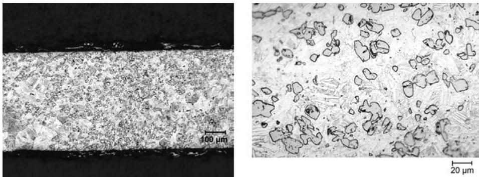
Fig. 8 Microstructure of titanium MMC strip produced by direct powder rolling plus sintering. Density is 4.25 g/cm<sup>3</sup>.
