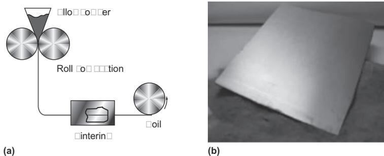
Fig. 10 (a) Schematic of Ametek roll compaction process and (b) roll-compacted sheet (Ref 16)
