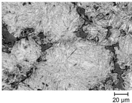
**Fig. 9** Tempered martensitic microstructure of a quench-hardened and tempered PM copper steel (FC-0208)
