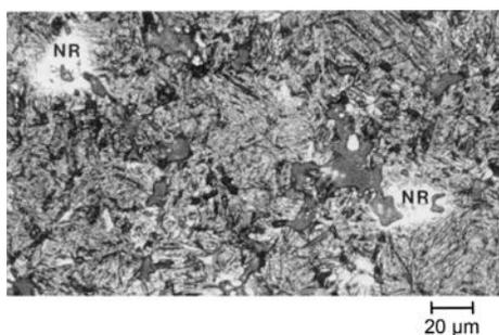
**Fig. 13** Nickel-rich regions (NR) in a tempered martensitic structure of a quench-hardened and tempered PM nickel steel (FN-0208)
