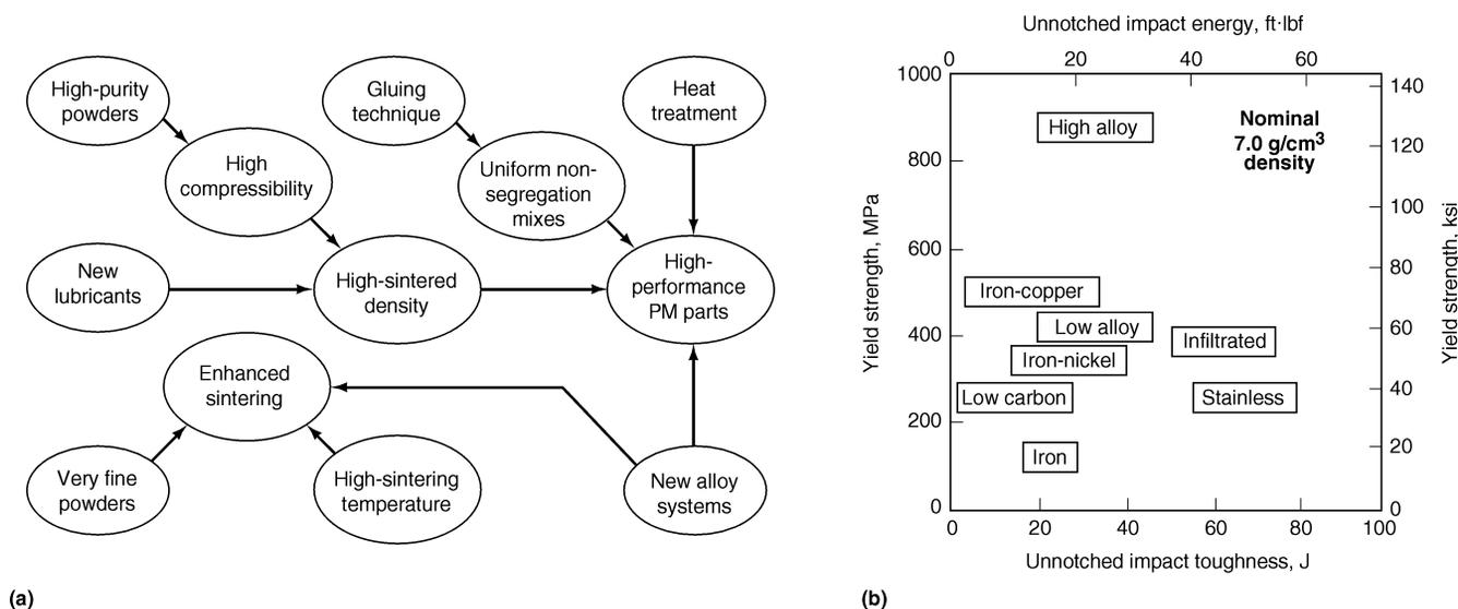
**Fig. 2** General methods to achieve high-performance PM steels. (a) Processing options. (b) Higher alloying to improve strength and toughness. Source Ref 2 and 3
