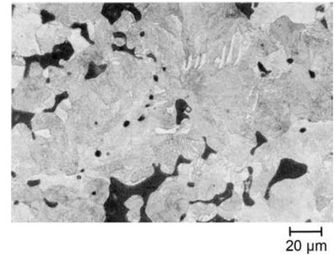
**Fig. 8** Ferrite-pearlite microstructure of an as-sintered PM copper steel (FC-0208)
