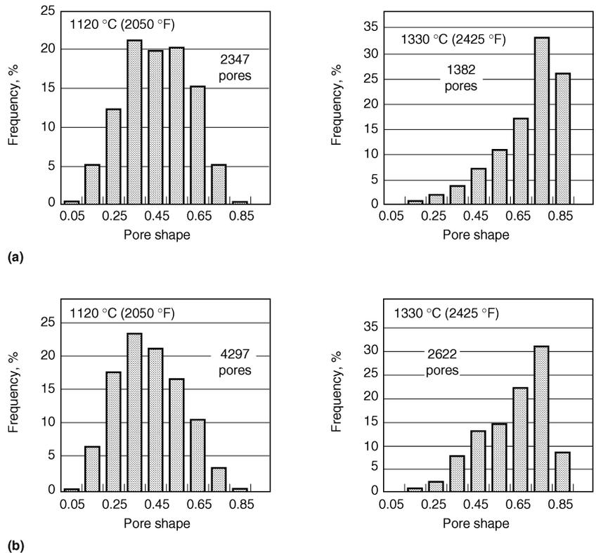
**Fig. 10** Shape and size of porosity in PM copper (FC-0208) and nickel (FN-0208) steels. Pore shape = 4nA/p<sup>2</sup> (for a circular pore = 1). Source: Ref 23
