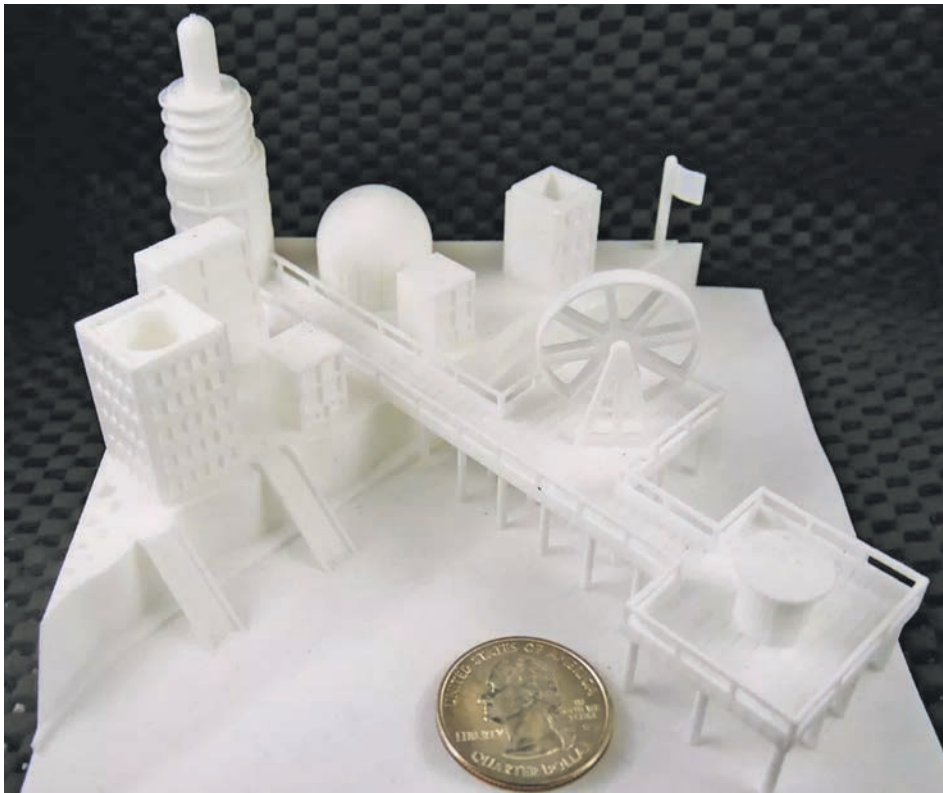
Fig. 12 Powder bed fusion part, nylon. Courtesy of 3D Systems
