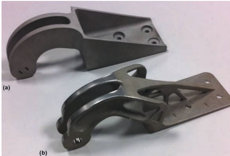
Fig. 3 Nacelle hinge bracket for Airbus A320 (a) and topology-optimized design produced by additive manufacturing (b). Courtesy of EADS and Altair (Ref 2,3)
