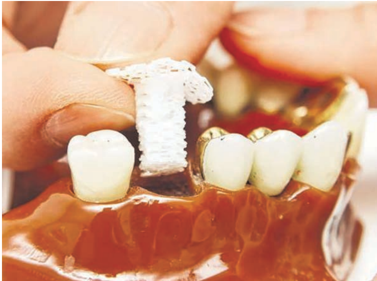
Fig. 4 Cellular bone scaffold for dental implantation. Courtesy of Nanyang Technological University
