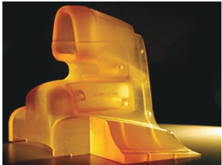
Fig. 8 Stereolithography wind tunnel part designed for Lotus Formula 1. Courtesy of 3D Systems (Ref 6)
