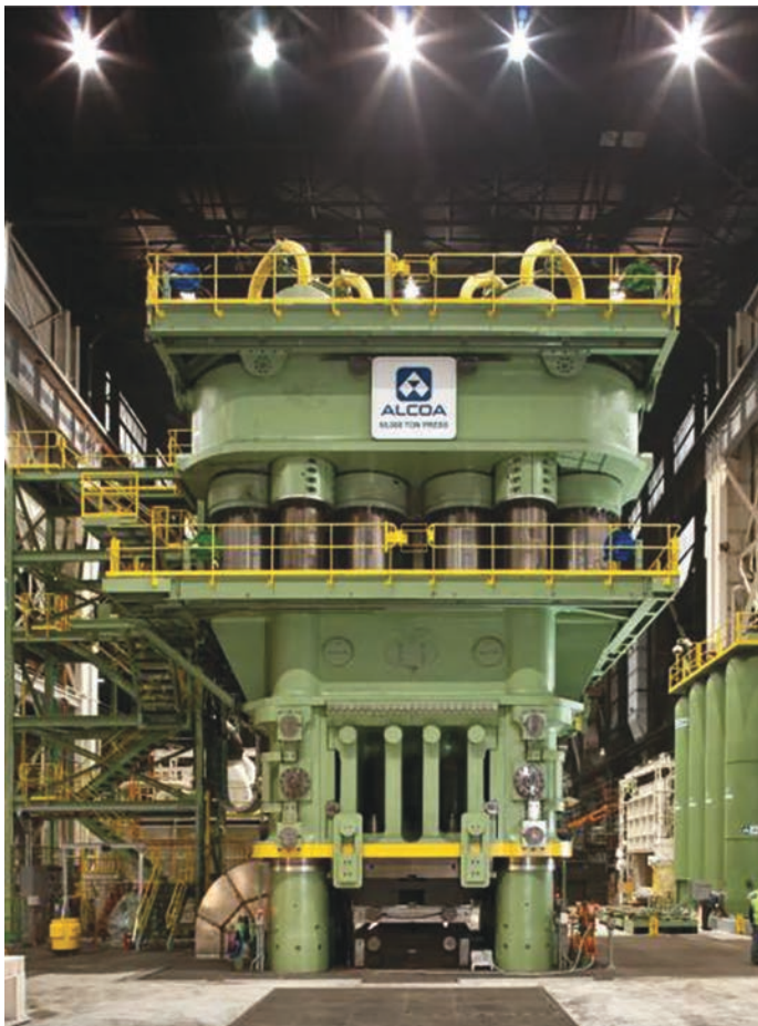
Fig. 15 A 50,000-ton hydraulic press at Arconic-Cleveland
