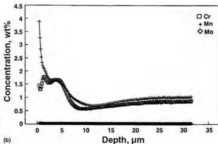
Fig. 6 Distribution of alloying elements close to the surface after (a) low-pressure carburizing and (b) atmospheric gas carburizing. Material is SAE 5115.
