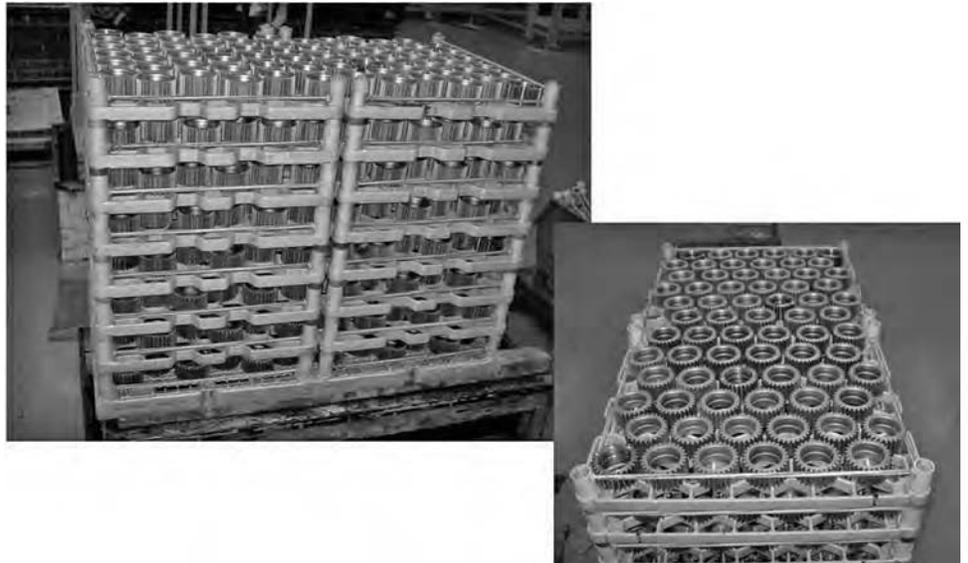
**Fig. 14** Load configuration for low-pressure carburizing of sun gears. 20MnCr5HH gear wheel; 576 parts per batch; cycle time, 215 min; carburizing temperature,  $945\text{ }^{\circ}\text{C}$  ( $1735\text{ }^{\circ}\text{F}$ ); nitrogen, 8 bar (6000 torr); case-hardening depth, 0.65–0.75 mm (0.026–0.030 in.); core hardness, 35–38 HRC
