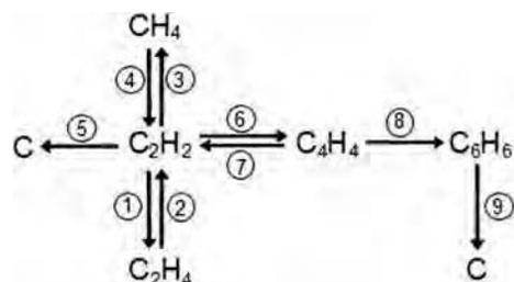
Fig. 4 Dissociation reactions during acetylene pyrolysis. Source: Ref 2
