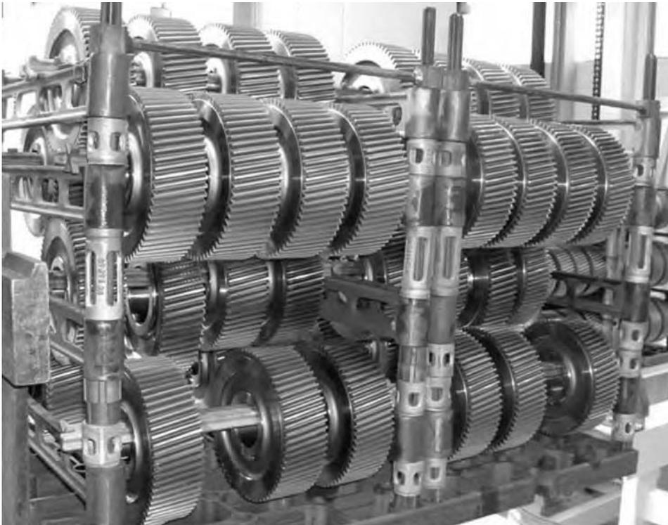
**Fig. 15** Load configuration for low-pressure carburizing of ring gears. 16MnCr5 gear wheel; 44 parts per batch; cycle time, 450 min; carburizing temperature, 930 °C (1705 °F); helium, 18 bar (13,500 torr); case-hardening depth, 0.85–0.95 mm (0.034–0.037 in.); core hardness, 27–30 HRC
