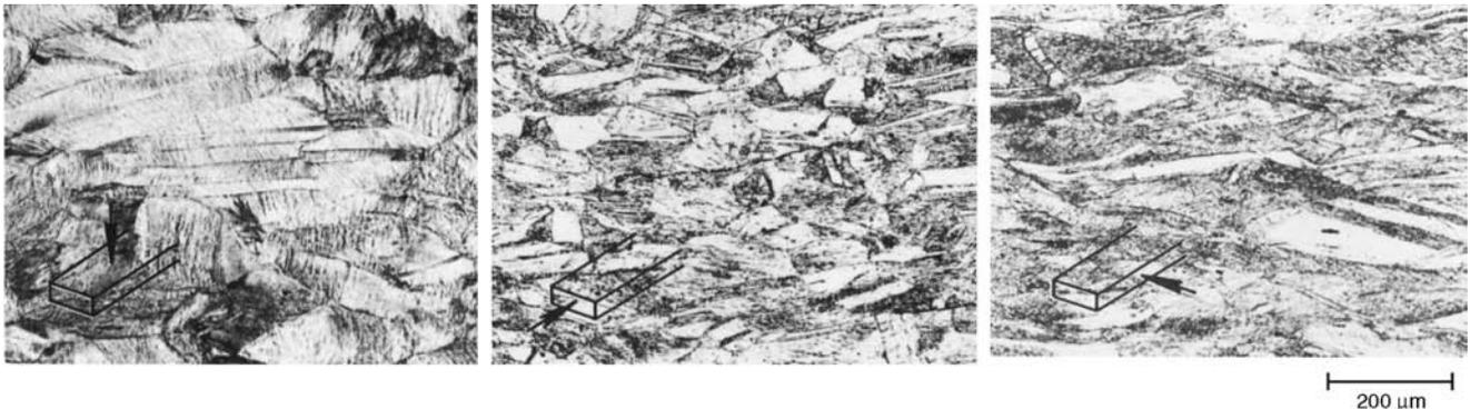
**Fig. 23** Same alloy and processing as in Fig. 22, but reduced 50% by cold rolling from 6 mm (0.239 in.) to 3 mm (0.120 in.). Grains are elongated in the rolling direction. Diagrams indicate same orientation of view as in Fig. 22. Etched using  $\text{NH}_4\text{OH}$  plus  $\text{H}_2\text{O}_2$ .  $75\times$ . Source: Ref 8
