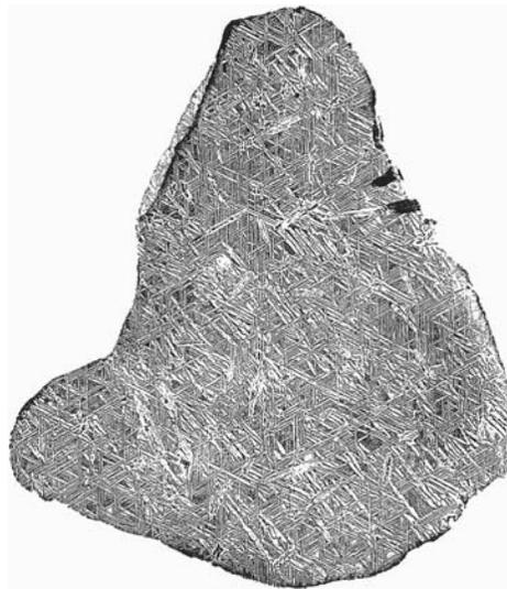
**Fig. 2** Macrograph of the Elbogen iron meteorite prepared in 1808 by Widmanstätten and Schreibers using heavy etching in nitric acid. After rinsing in water and drying, printer's ink was rolled on the etched surface, and the sample was pressed onto a piece of paper. Source: Ref 4
