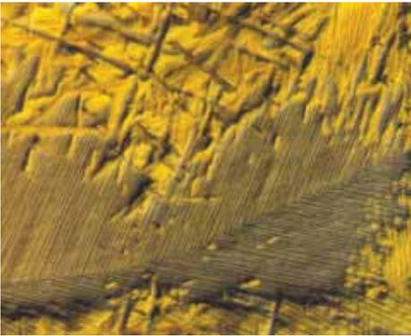
**Fig. 26** Zircaloy forging as viewed under differential interference contrast illumination. The parallel platelet structure is an area lower in carbon content. Etched in 45 mL H<sub>2</sub>O, 45 mL HNO<sub>3</sub>, and 10 mL HF and heat tinted at 425 °C (800 °F). 100×. (P.E. Danielson)
