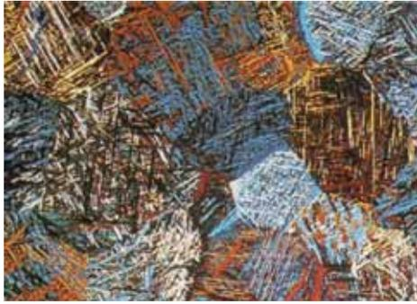
**Fig. 18** Ti-6Al-4V alloy containing martensite needles formed at elevated temperature ( $>840$  °C, or 1540 °F). Color etched in 100 mL  $H_2O$ , 4 mL HCl, 3 g  $NH_4HF_2$ . Polarized light illumination. 100 $\times$ . (G. Müller)
