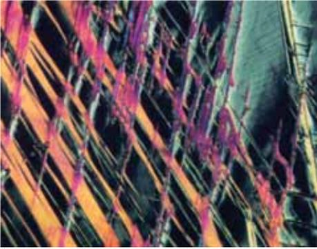
**Fig. 23** Hafnium crystal bar showing twins caused by cold working. Attack polished, heat tinted at 480 °C (900 °F), and viewed under differential interference contrast illumination. 65×. (P.E. Danielson)
