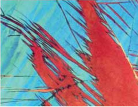
**Fig. 14** Mechanically twinned hafnium weld. Specimen was attack polished and heat tinted (~400 °C, or 750 °F). Polarized light illumination. 60×. (P.E. Danielson)
