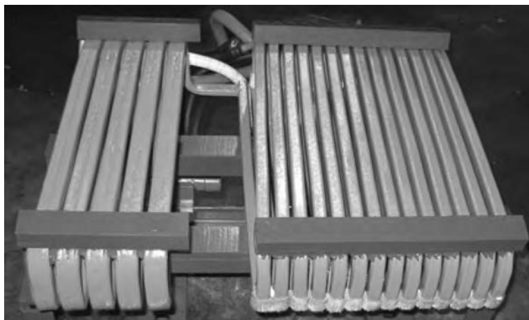
Fig. 9 Induction forge coil electrical insulation
