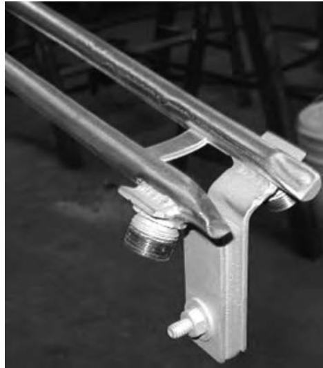
Fig. 23 Coated water-cooled wear rail. Courtesy of Ajax Tocco Magnethermic
