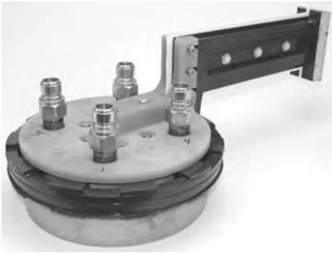
Fig. 2 Example of an inside diameter heat treating coil with quench follower. Flux concentrators and a machined profile on the current-carrying face control the shape of the hardened area. Brazing coils typically do not require machined profiles, because the heated area usually does not need to be as sharply defined as in heat treating. Courtesy of Radyne Corporation, an Inductotherm Group Co.
