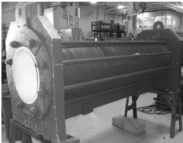
Fig. 13 Low-frequency coil design in which the induction coil winding is compressed between end plates
