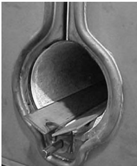
Fig. 27 Typical installation of the end of a hot rail installed in a round induction coil. Courtesy of Pillar Induction
