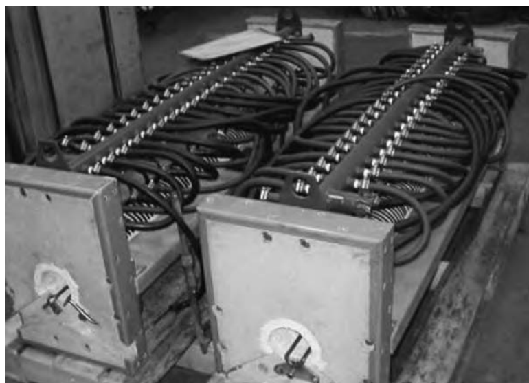
Fig. 17 Two billet-heating coils that feature the cast refractory end plates with fiberglass channel installed around the outside perimeter. Courtesy of Pillar Induction
