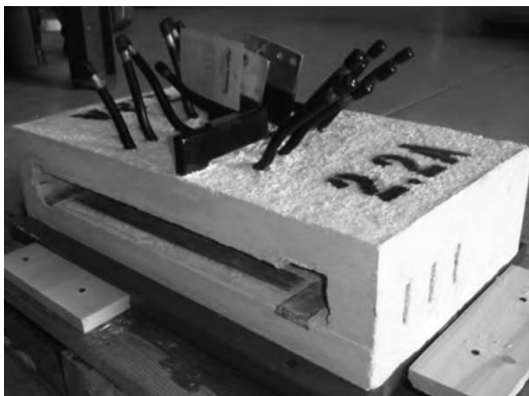
Fig. 29 Induction coil designed with silicon nitride trapezoid wear rails that are embedded into the surface of the refractory, with approximately 1.6 mm ( \frac{1}{16} in.) raised above the surface. The rails are used in both the entrance and exit ends as well as across the center of the induction oval-style coil in two areas where the bars are conveyed across the surface. Courtesy of Ajax Tocco Magnethermic
