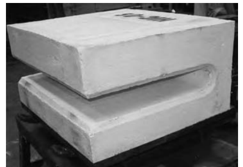
Fig. 15 Monolithic all-cast channel or conveyor coil typically used to heat bar ends for warm and hot forging applications. Courtesy of Ajax Tocco Magnethermic
