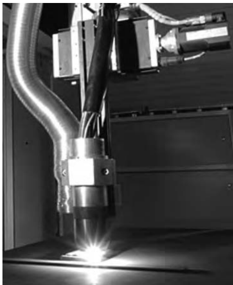
Fig. 26 Plasma-transferred arc process used to apply a wear bead to a rail
