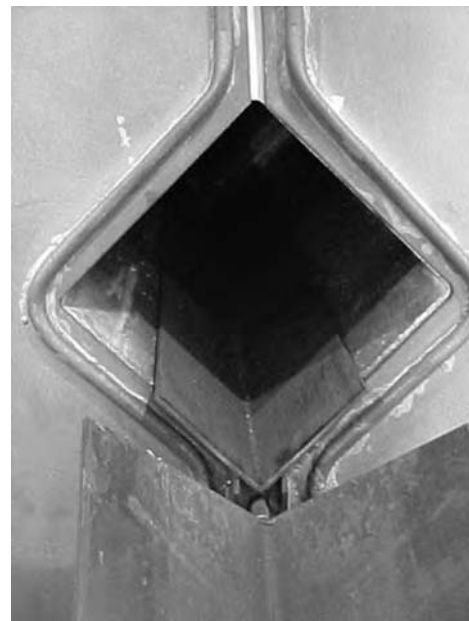
Fig. 28 Typical installation of the end of a hot rail installed in a round-cornered square induction coil. Courtesy of Pillar Induction
