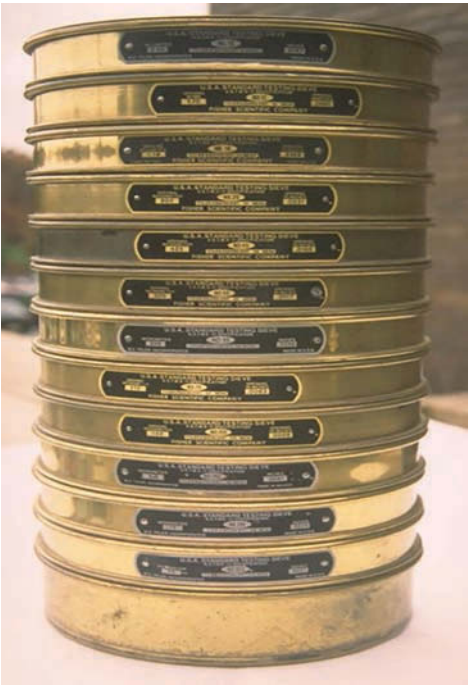
Fig. 30 Sieves stacked in a series from large openings (top) to small openings (bottom) to monitor abrasive breakdown
