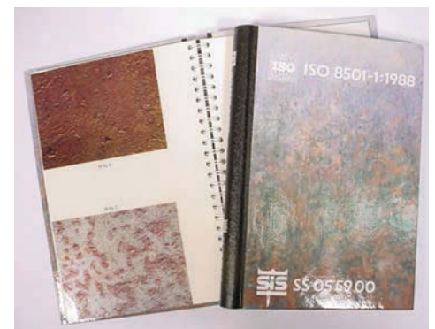
Fig. 43 ISO 8501-1 visual guide for surface-cleanliness evaluations
