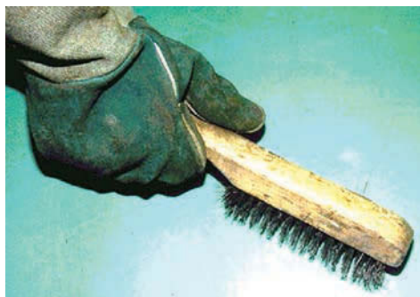
Fig. 21 Wire brush used to perform hand tool cleaning
