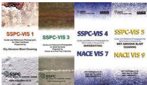
Fig. 41 The SSPC visual guides for surface-cleanliness evaluations
