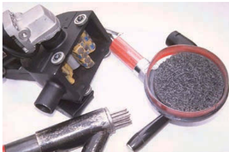
Fig. 23 Rotating flap, needle scaler, and nonwoven fiber wheel used to perform power tool cleaning
