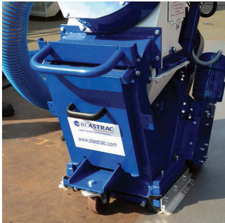
Fig. 28 Portable centrifugal abrasive blast machine. Photo used with permission from BlasTrac
