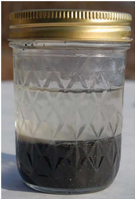
Fig. 31 Vial test for abrasive cleanliness
