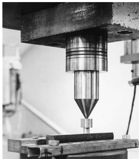
Fig. 7 Button-on-block galling test arrangement using a tension test machine. Source: Ref 16
