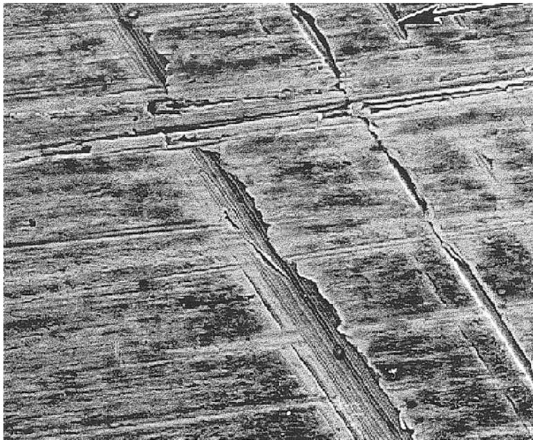
Fig. 3 SEM micrograph of adhesive wear of cast iron
