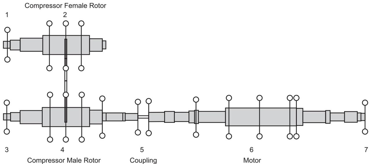
**Figure 4-29—Typical System Model of a Flooded Compressor Train**
