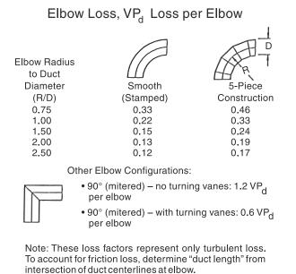
FIGURE 8-1. Elbow pressure loss for round duct elbows. (Source: ACGIH Industrial Ventilation Manual<sup>(1)</sup>)
