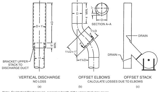
Note: For Vertical Discharge (a), excessive length of the upper stack may cause "blowout" of discharged air at the gap between the upper and lower sections.
