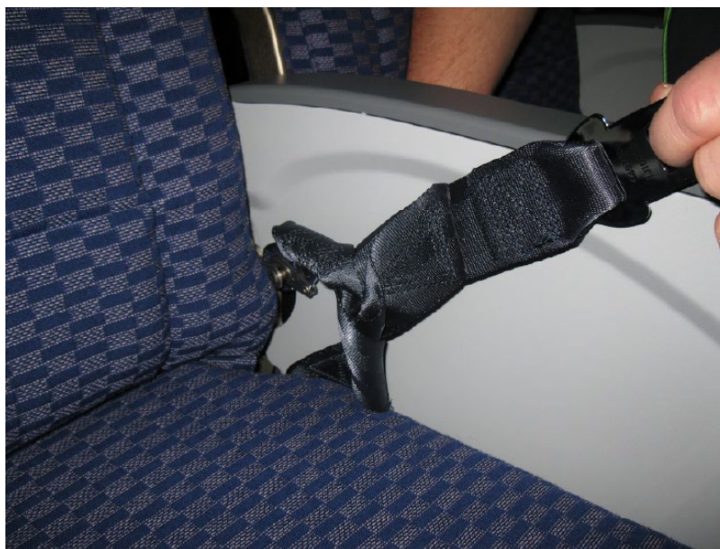
Figure 7 - Seat Y-belt misalignment
