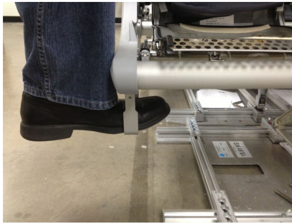
Figure 27 - Acceptable foot insertion into stirrup-type step
