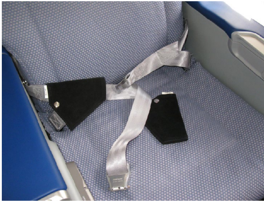
Figure 8 - Belt cover non-permanent attachment
