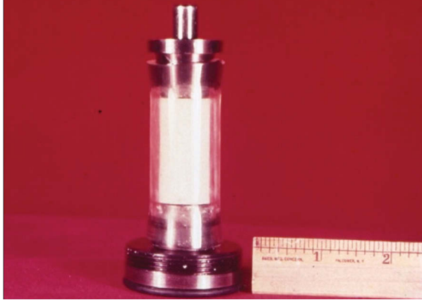
Figure 5-4: Jacketed sample of rock ready for testing.
