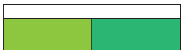
Figure 12-40: After dilution, the drilling fluid once again contains only 100 bbl of drilled solids for the 2,100 bbl.
