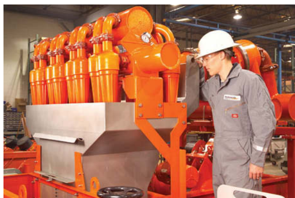
Figure 12-12: Commercially available mud cleaners. Top: Derrick Dual Pool 600 Shaker with Mud Cleaner Option. Courtesy Derrick Equipment Company. Bottom: M-I SWACO mud cleaners combine a hydrocyclone system with a shale shaker and are designed to process the entire drilling fluid circulating volume. Courtesy Schlumberger.
