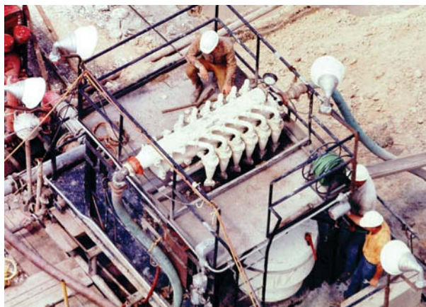
Figure 12-11b: A second field test was followed by one at Tilden, Texas, using potassium chloride drilling fluid. The mud cleaner removed detrimental drilled solids and also recovered a significant quantity of expensive drilling fluid.
