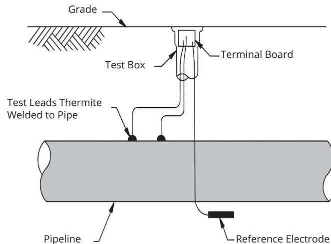
Figure 10-19 Corrosion monitoring station
