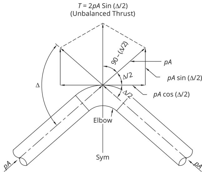
Figure 8-7 Unbalanced thrust at horizontal bends,  $T = 2pA \sin \Delta/2$
