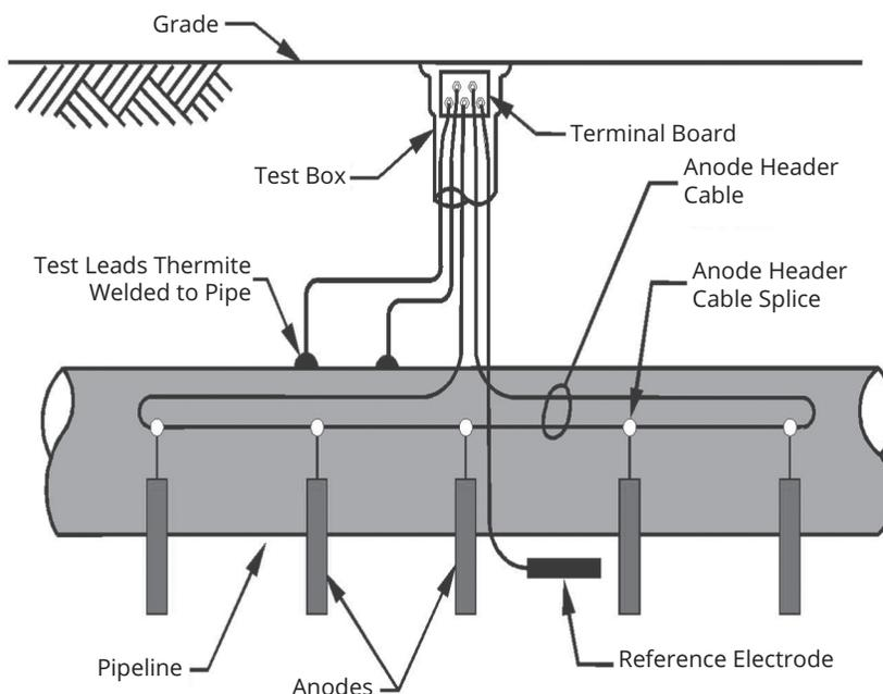
Figure 10-20 Galvanic anode cathodic protection
