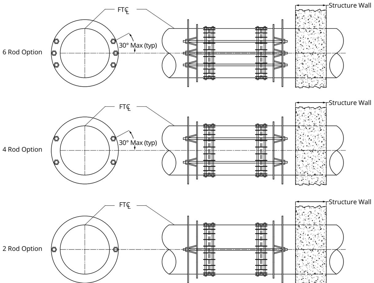
**Figure C-1** Harness rod placement for differential settlement across multiple harnessed joints (section view)
