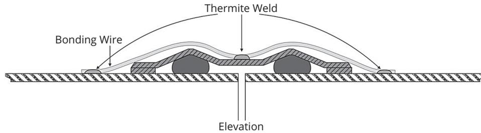
Figure 10-18 Bonding wires installed on split-sleeve-type coupling
