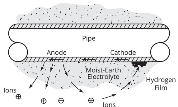
Moist earth is the electrolyte; two areas on the uncoated pipe are anode and cathode; pipe wall takes the place of wire in Figures 10-2 and 10-4. Pipe wall at anode will corrode like the zinc battery case; pipe wall at cathode site will not corrode but will tend to be protected as polarization develops and if not removed, will tend to build resistance to current flow and thereby eliminate or slow the corrosion of pipe wall at anode site. Coatings prevent cell formation.
