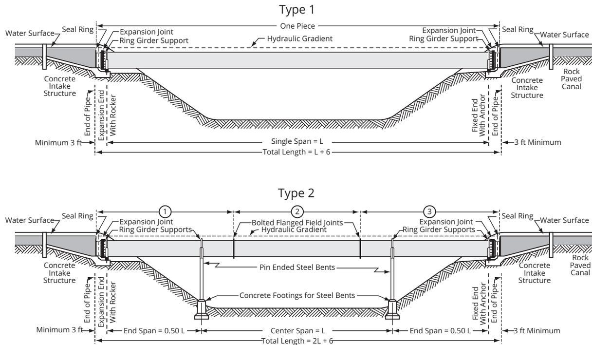
Figure 9-6 Long-span steel pipe for low pressures
