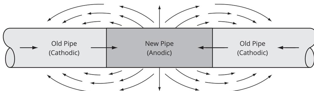
Although seldom considered, a galvanic cell is created by installing a piece of new uncoated pipe in an old line. New pipe always becomes the anode, and its rate of corrosion will depend on type of soil and relative areas of anode and cathode. Therefore, corrosion protection measures are essential.
