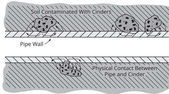
When uncoated metal pipe is laid in cinders, corrosive action is that of dissimilar metals. Cinders are one metal (cathode) and pipe the other (anode). Acid leached from cinders contaminates soil and increases its activity. No hydrogen collects on the cinder cathode, the cell remains active, and corrosion is rapid.
