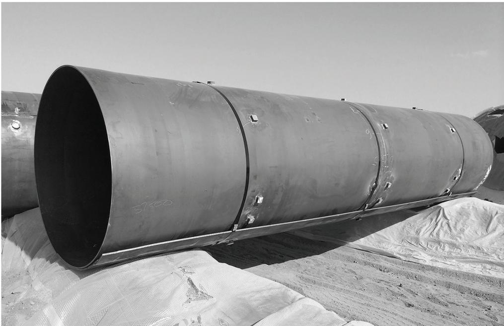
Figure 12-2 Steel reliner section
