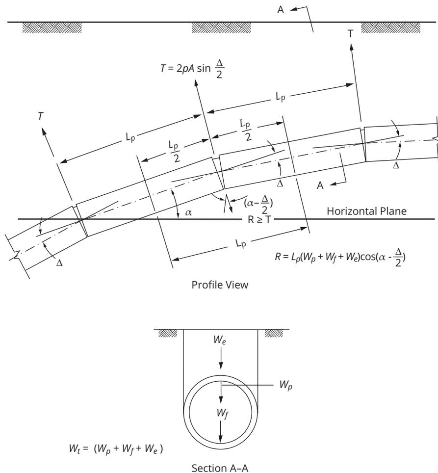
Figure 8-9 Restraint of uplift thrust at deflected joints on long-radius vertical curves
