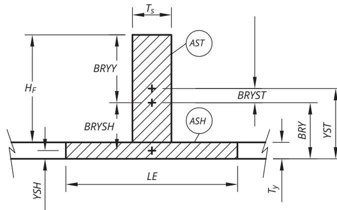
Figure B-3 Front harness ring/shell section
