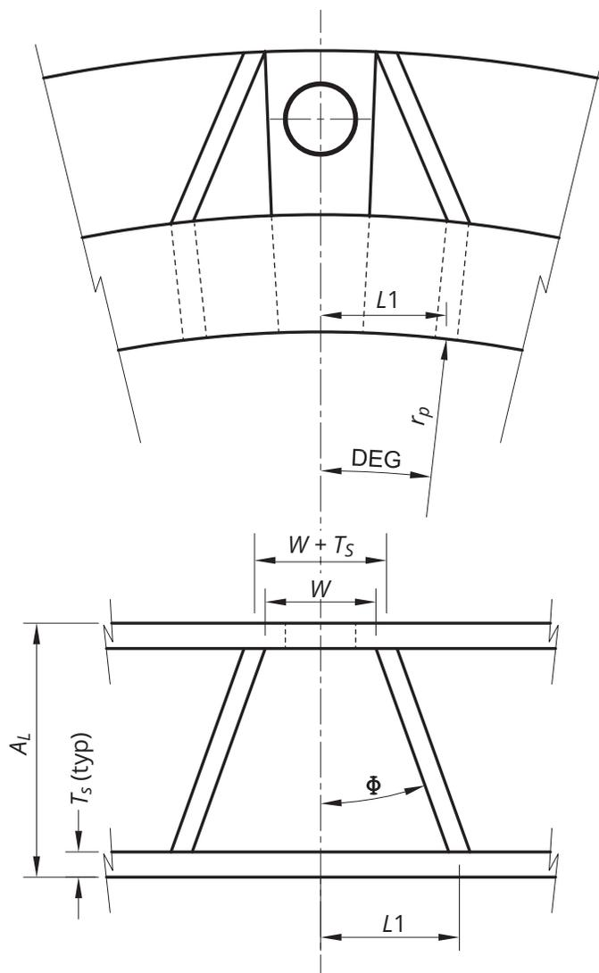
Figure B-1 Harness lug geometry
