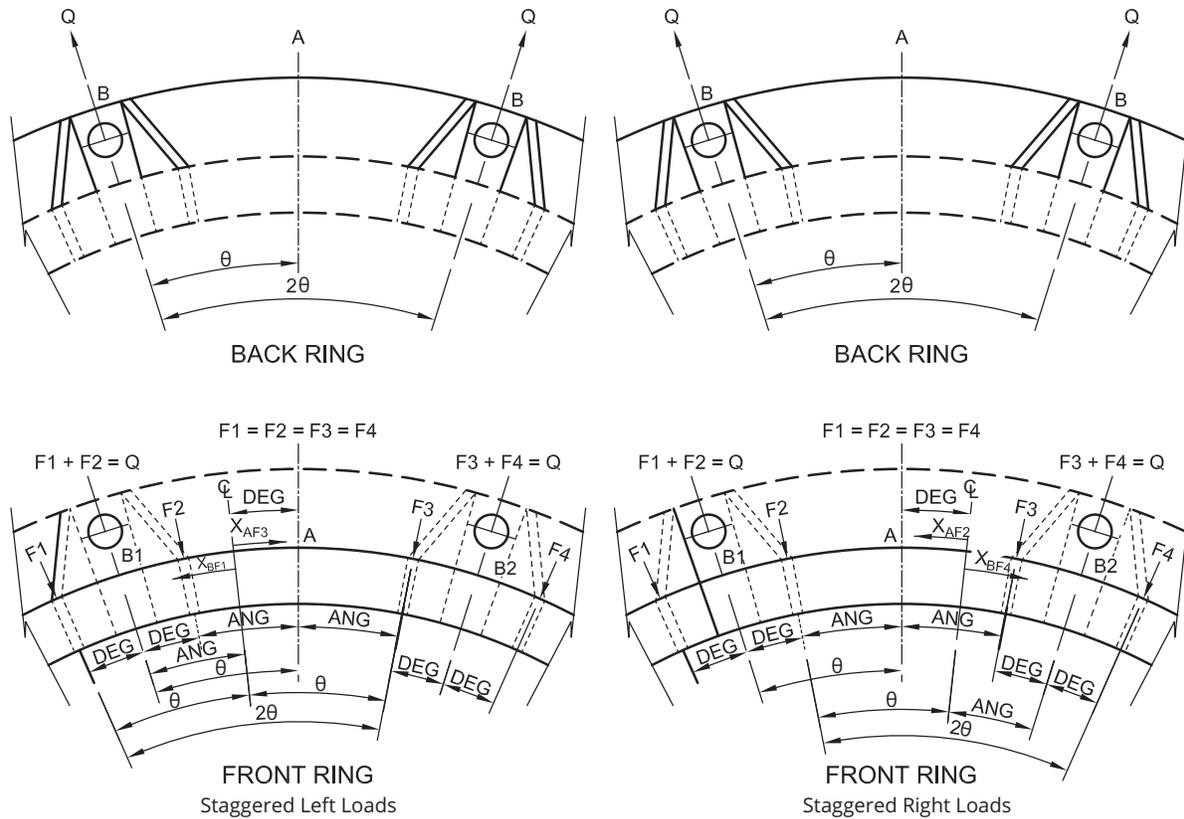
Figure B-2 Harness lug assembly geometry
