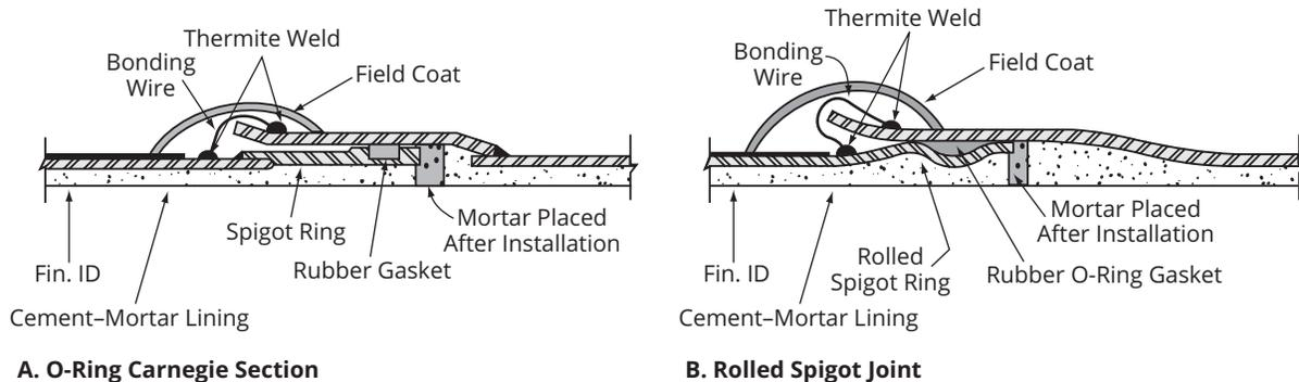
Figure 10-16 Bonding wire for bell-and-spigot rubber-gasketed joint
