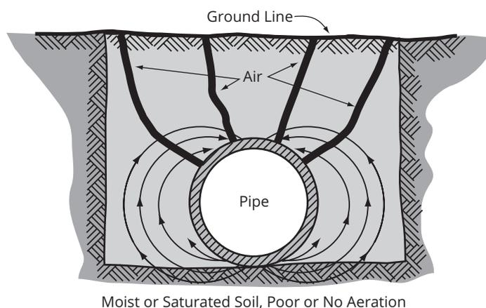
This is another galvanic cell of dissimilar-electrolyte type. Soil throughout the depth of the excavation is uniform, but a portion of the pipe rests on heavy, moist, undisturbed ground at the bottom of the excavation, while the remainder of the uncoated pipe is in contact with drier and more aerated soil backfill. Greatest dissimilarity—and the most dangerous condition—occur along a narrow strip at the bottom of the pipe, which is the anode of the cell.
