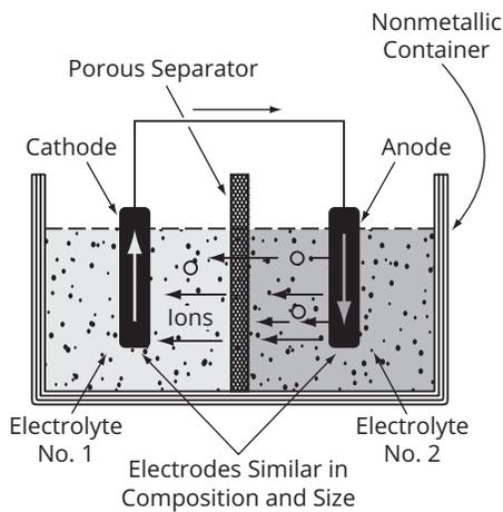
Figure 10-4 Corrosion cell—dissimilar electrolytes typical of car battery
