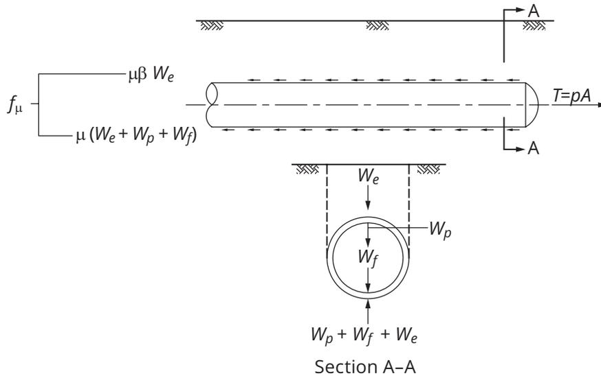
Figure 8-4 Horizontal frictional forces that resist horizontal thrust  $T = pA$
