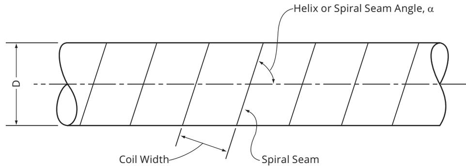
**Figure E-4 Spiral pipe helix angle**
