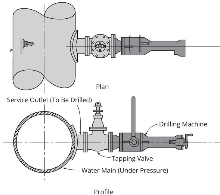
Procedure: (1) Weld outlet and reinforcing collar (if required) to main; (2) bolt on gate valve, adapter (if required), and drilling machine; (3) insert tool and drill hole in main; and (4) withdraw tool, close gate, and remove machine.
