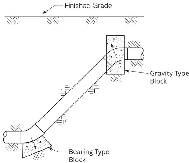
Figure 8-3 Typical thrust blocking of vertical bends with bearing-type and gravity-type blocks
