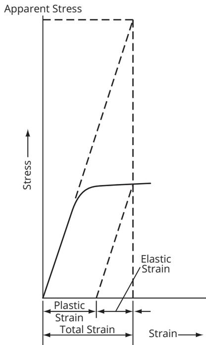
If the total strain is multiplied by the modulus of elasticity, the stress determined by use of a formula based on Hooke's law is fictitious.
