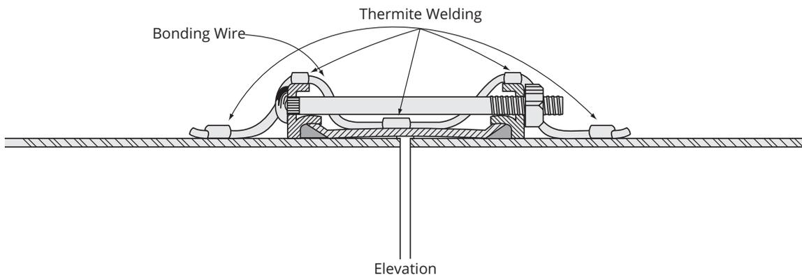
Figure 10-17 Bonding wires installed on sleeve-type coupling
