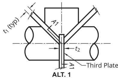
(See two plate connection details for welding alt. 1 based on integral or external connection)
