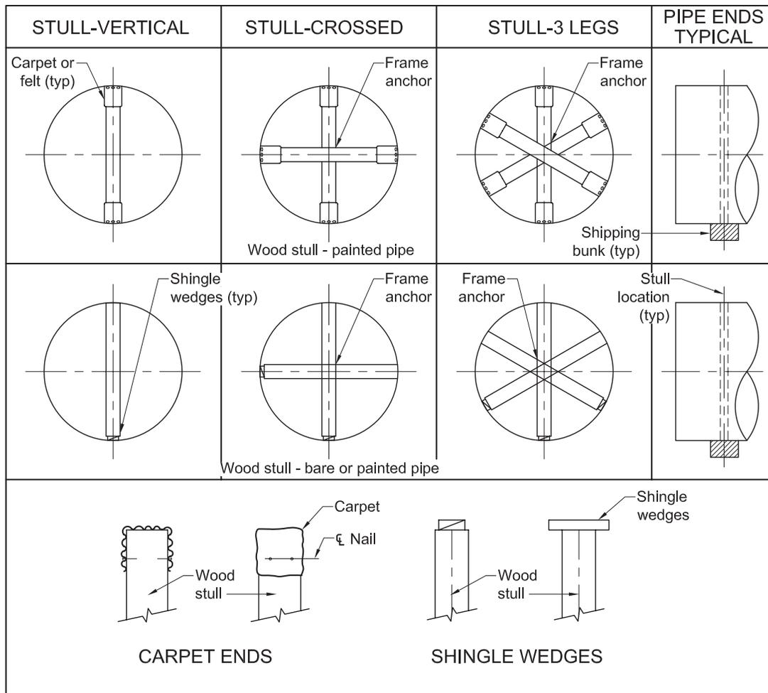
Figure 12-1 Pipe stulling and bracing configurations
