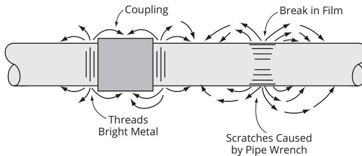
Bright scars or scratches of threads become anode areas in buried pipe, and the rest of the pipe is a cathodic area. In some soils, these bright areas can be very active and destructive because the small anode area and large cathode area produce the most unfavorable ratios possible.
