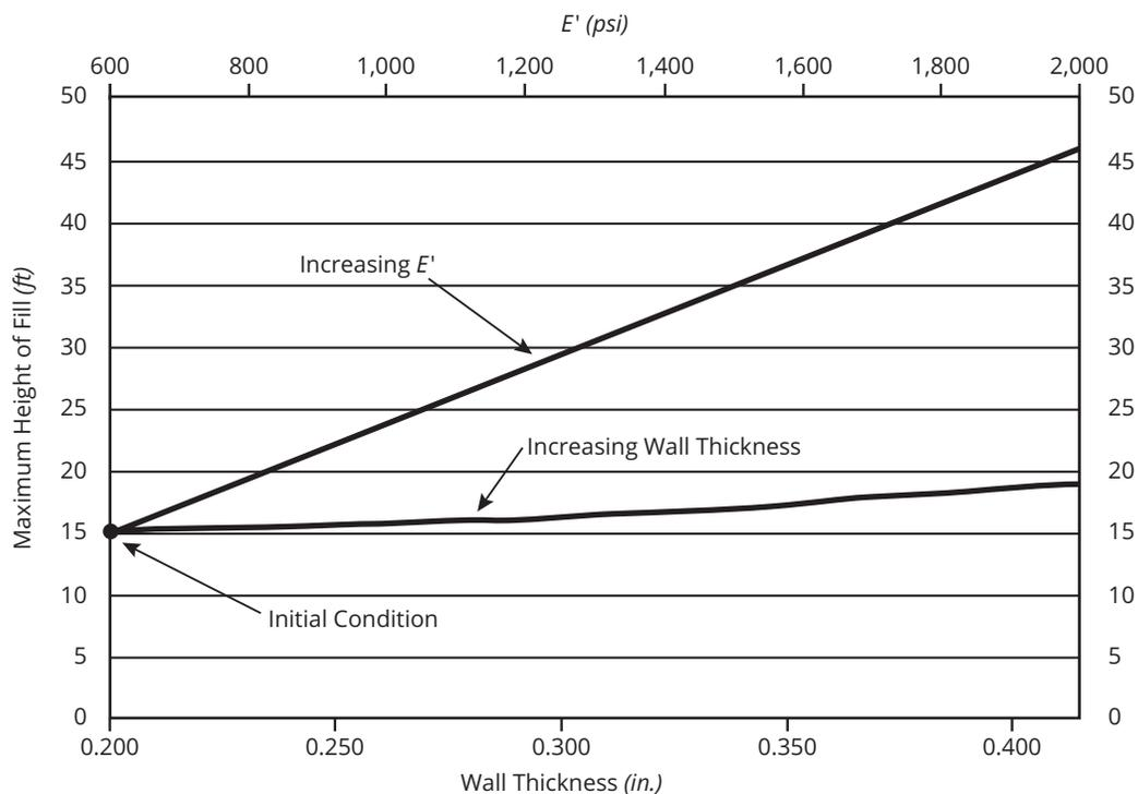
Figure A-1 Comparison of improving pipe embedment versus increasing wall thickness for 48-in. pipe
