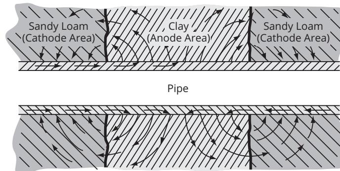
In this corrosion cell of dissimilar electrolytes (compare Figure 10-3), sections of uncoated pipe in sandy loam are cathodes (protected areas), sections in clay are anodes (corroding areas), and soil is electrolyte. If resistance to electric-current flow is high in the electrolyte, the corrosion rate will be slow. If resistance to current flow is low, corrosion rate will be high. Thus, knowledge of soil resistance to electric-current flow becomes important in corrosion protection studies.
