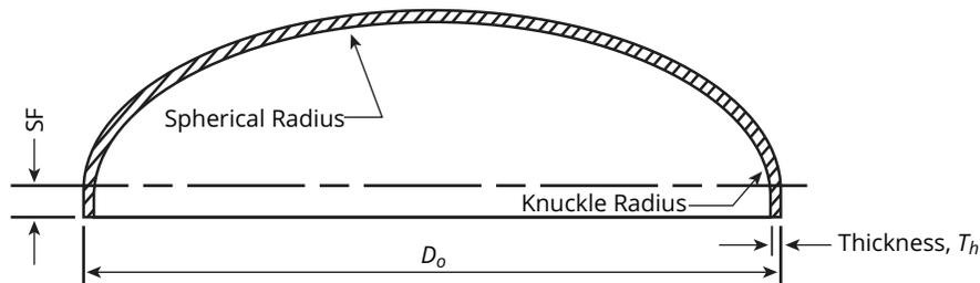
Figure 7-24 Approximation of an ellipsoidal head
