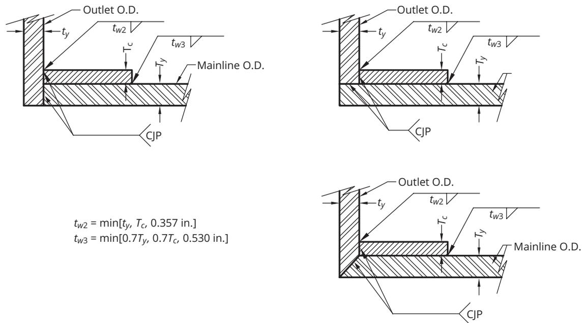
Figure 7-8 Configurations and welding for outlet requiring reinforcement
