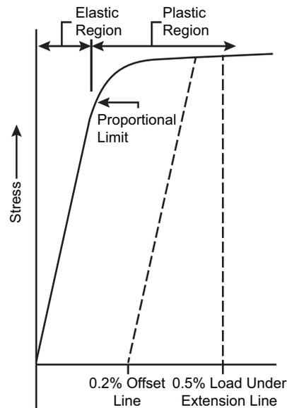
Shown are the elastic and plastic portions of a stress-strain curve. Note: the 0.2% and 0.5% lines intersect at a specific location that may not be located on the stress-strain curve.
