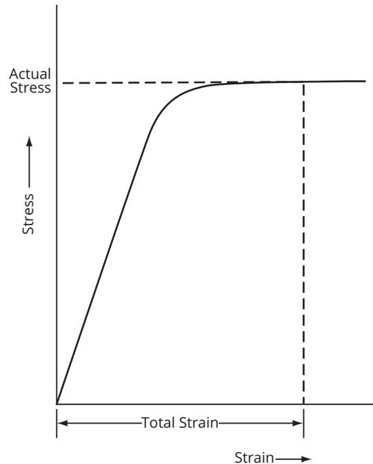
When the total measured strain is known, the actual stress can be determined by use of the stress-strain curve.
