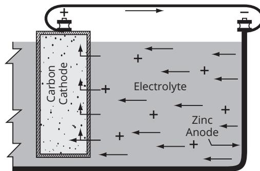
Figure 10-2 Electrochemical corrosion cell—alkaline flashlight battery
