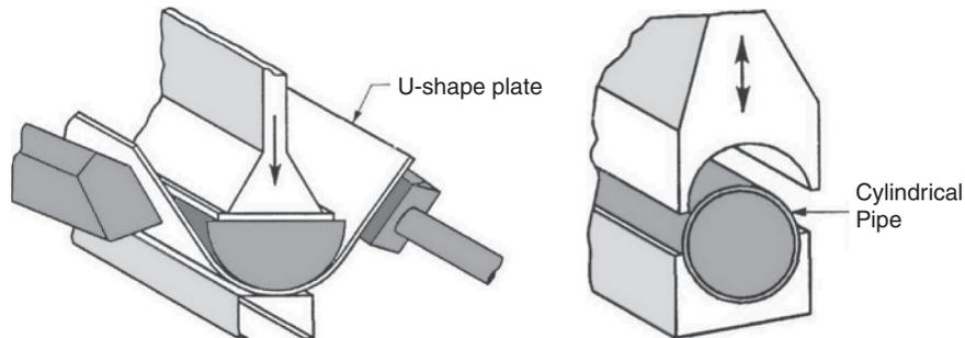
Figure 2-2 U-ing and O-ing straight-seam double-fusion-welded pipe
