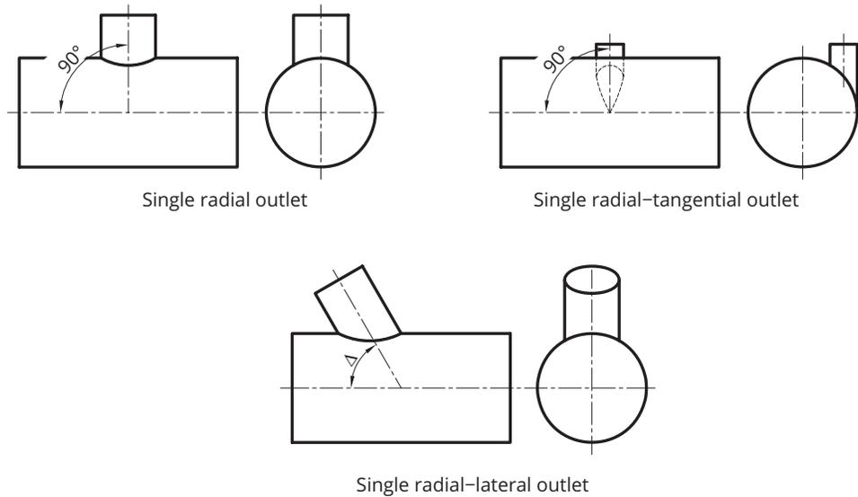
Figure 7-3 Common outlet configuration terminology
