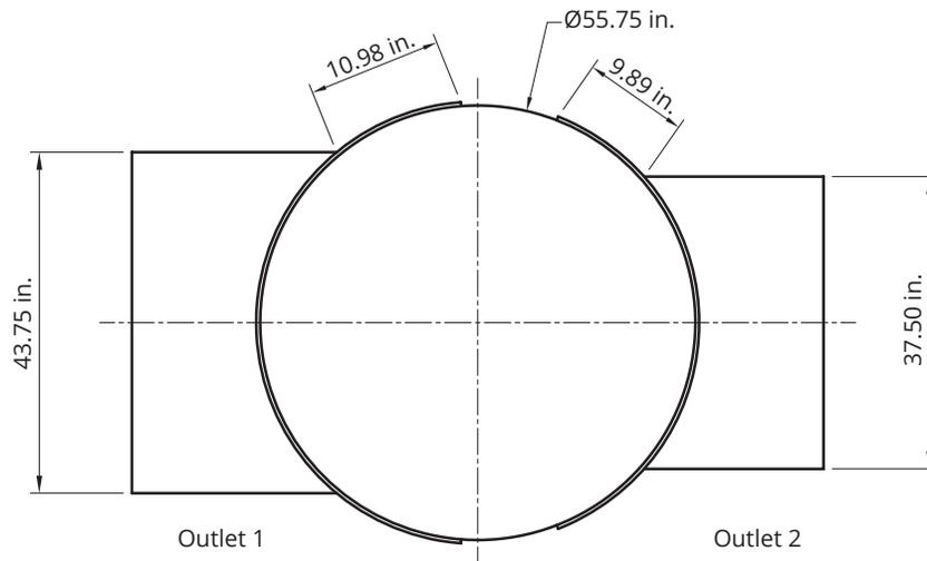
Figure 7-6 Scale drawing of the resulting geometry of double outlet
