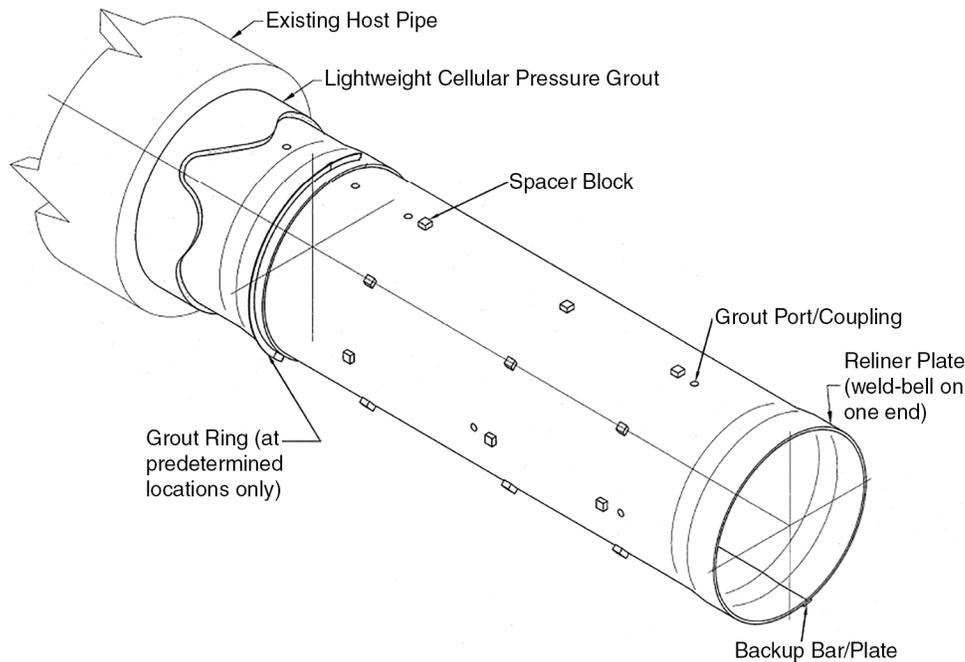
Figure 12-3 Steel reliner assembly view (not to scale)
