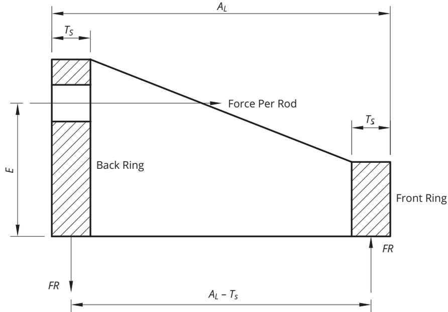
Figure B-5 Simplified lug free body diagram
