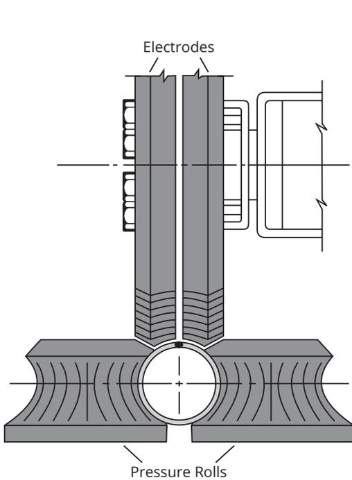
Application of pressure by rolls on both sides and beneath the electrodes forces the heated tube edges together to form a weld.
