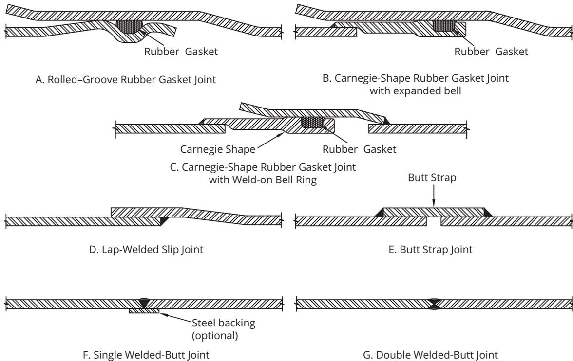
Figure 6-1 Common pipe field joints: Bell-and-spigot rubber gasket joints (A, B, and C) and field-welded joints (D–G)
