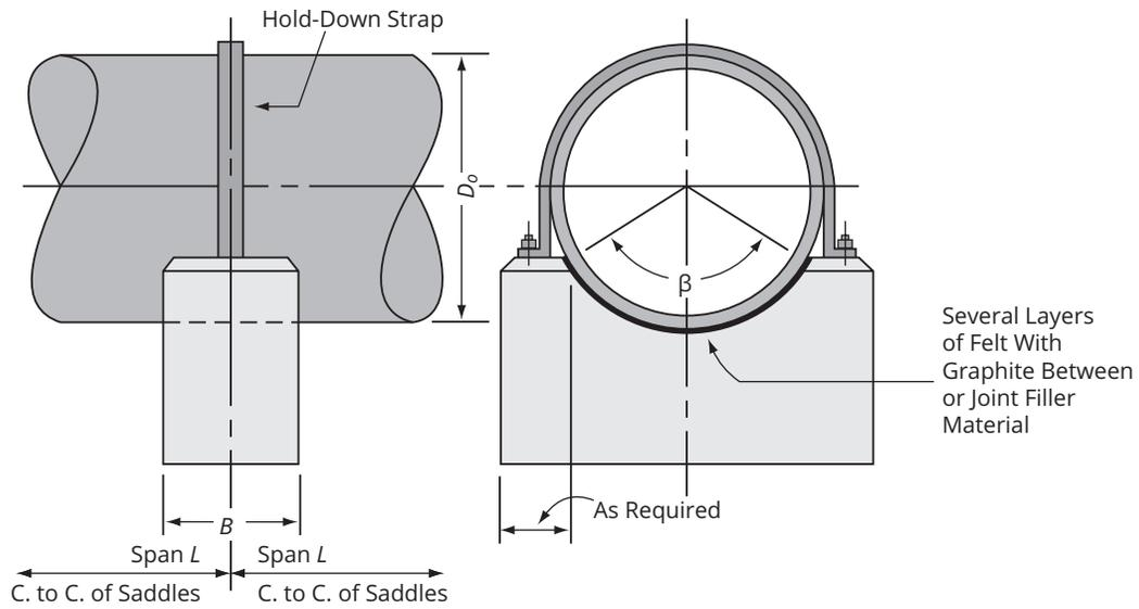
Pipe acting as a self-supporting bridge may rest on suitably padded concrete saddles.
