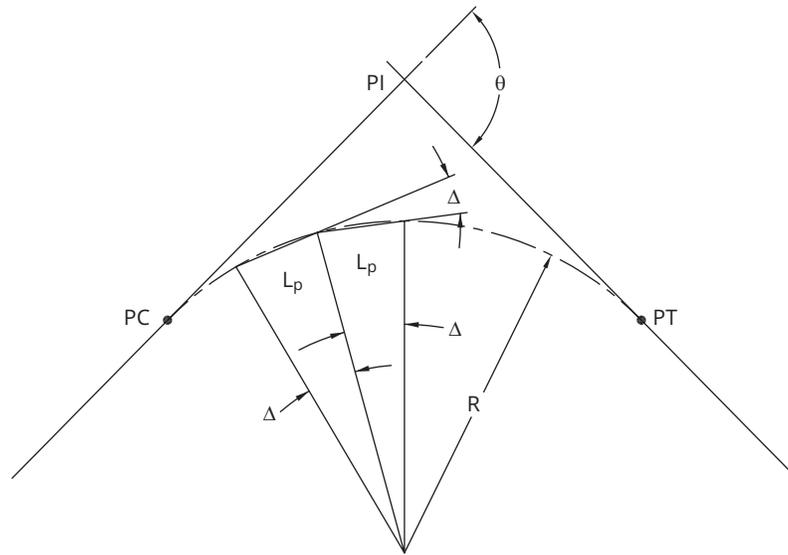
**Figure E-3 Pipe with deflected joints or mitered ends in a long-radius curve**
