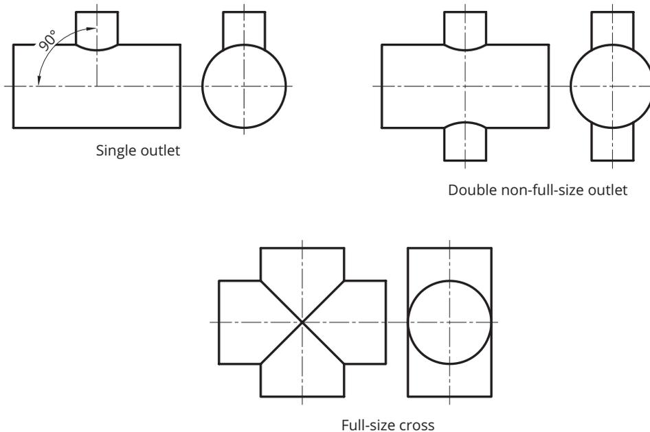
Figure 7-2 General outlet configurations
