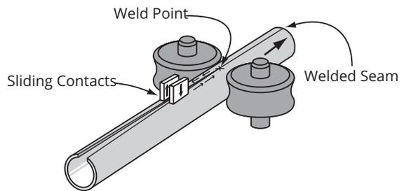
The current enters the tube via sliding contacts and flows along Vee edges to and from weld point.
