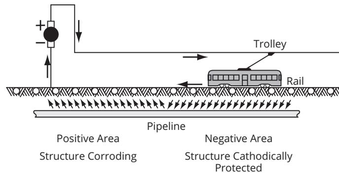
Figure 10-15 Stray-current corrosion caused by electrified railway systems
