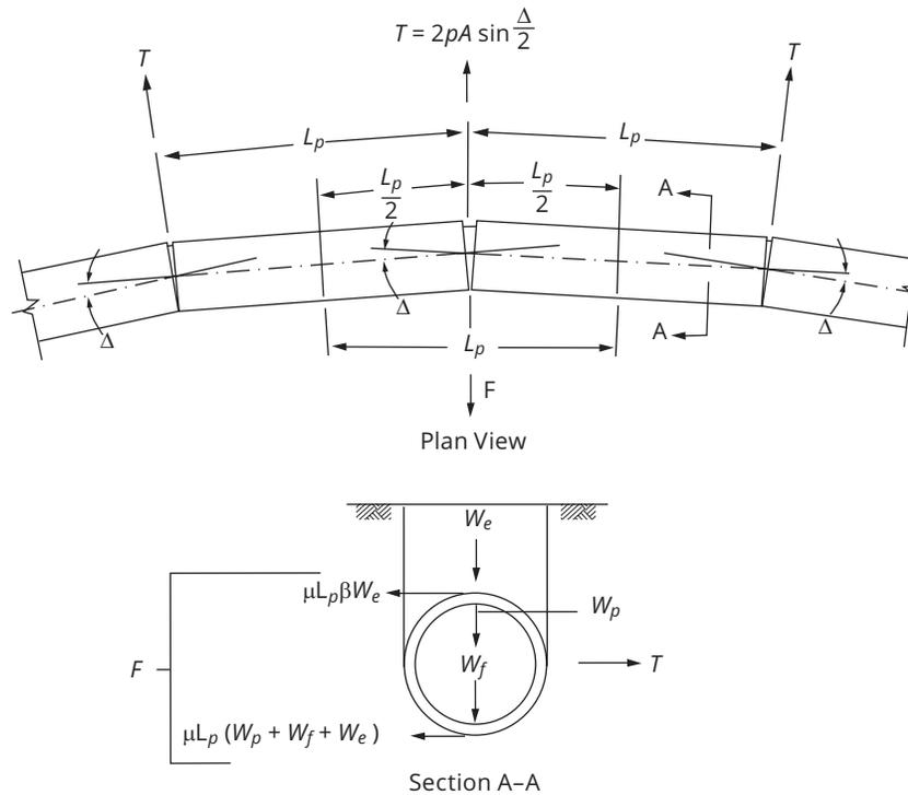
Figure 8-6 Restraint of thrust at deflected gasketed joints on long-radius horizontal curves
