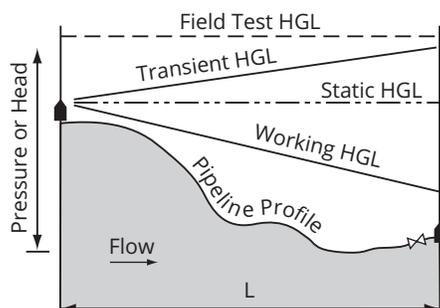
Figure 4-1 Typical pipeline and hydraulic grade profiles for gravity flow
