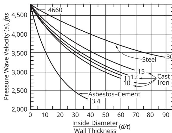
Note: The number at the end of each curve represents the modulus of elasticity ( $E$ ) in 1,000,000-psi units for various pipe materials.
