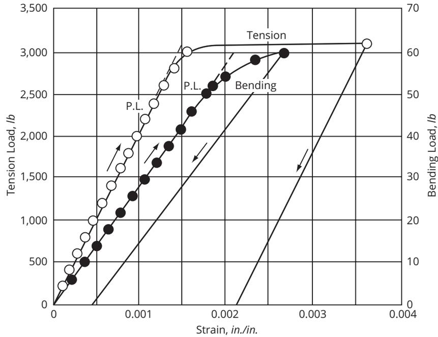
The proportional limit (P.L.) strains in bending are 1.52 times those in tension for the same material.
