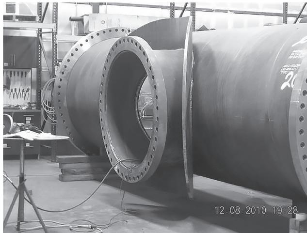
Figure 7-19 Illustration of one-plate design
