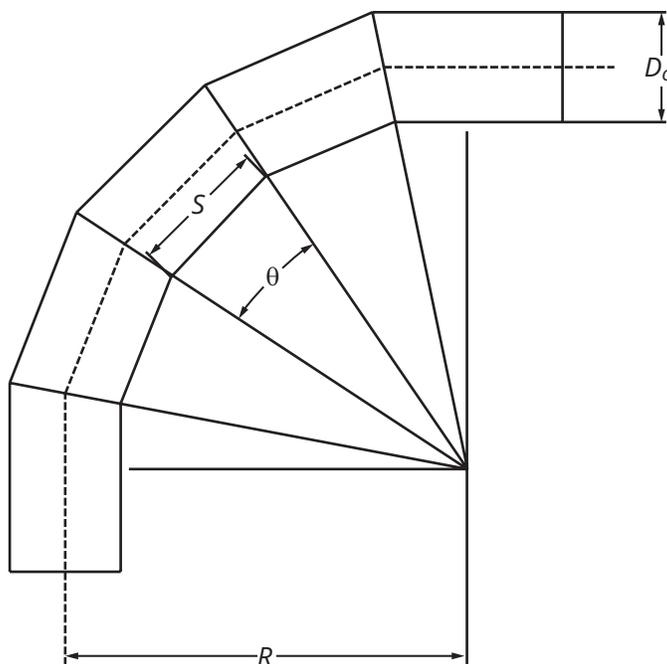
Figure 7-1 Basic elbow dimensions
