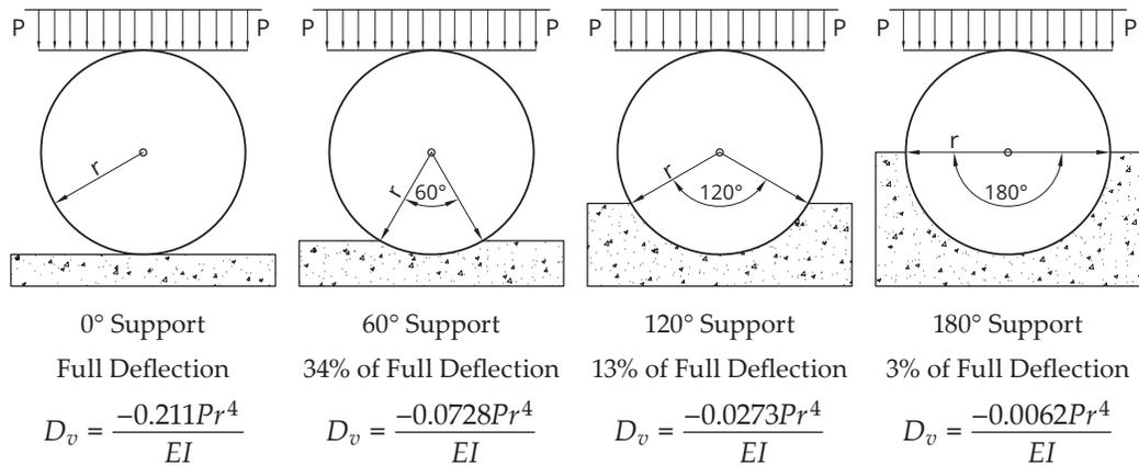
**Figure E-7 Various ring deflections of a circular ring under load with rigid bottom arc and no side support**
