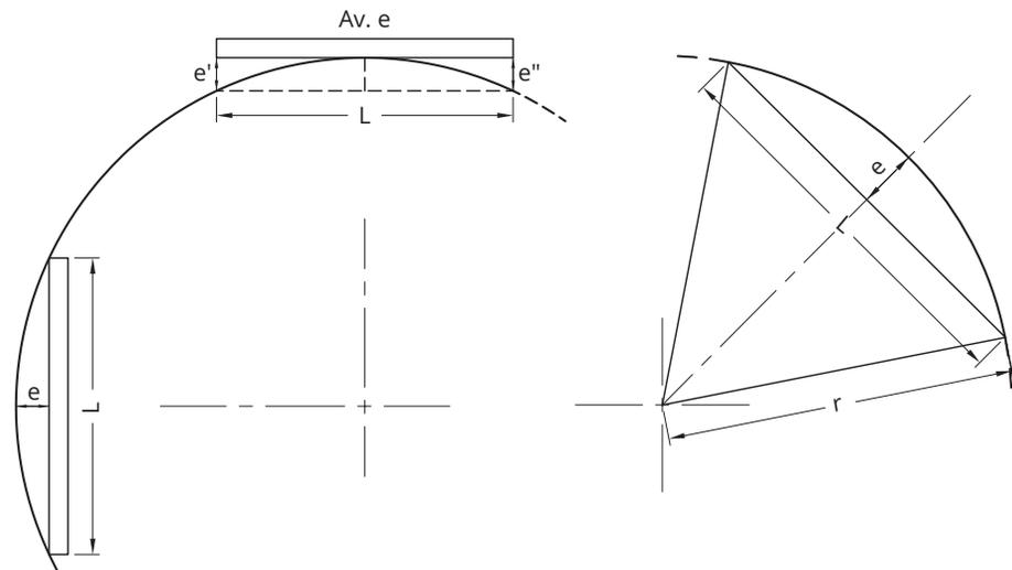
**Figure E-2 Measuring radius of curvature**
