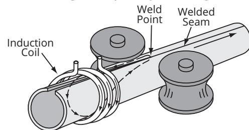
Eddy current flows around the back of the tube and along the edges to and from the weld point.
