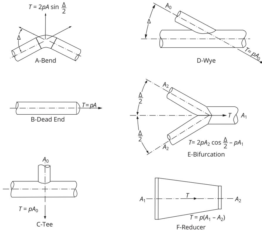
Figure 8-1 Hydrostatic thrust  $T$  applied by fluid pressure to typical fittings
