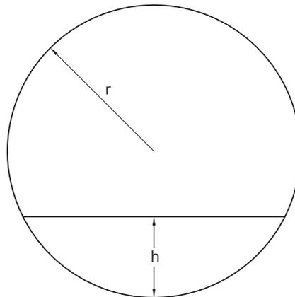
Figure E-1 Cross-section area of partially full cylinder
