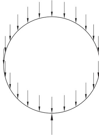
**Figure E-5 Vertical deflection of a pipe under its own weight on a flat surface**
