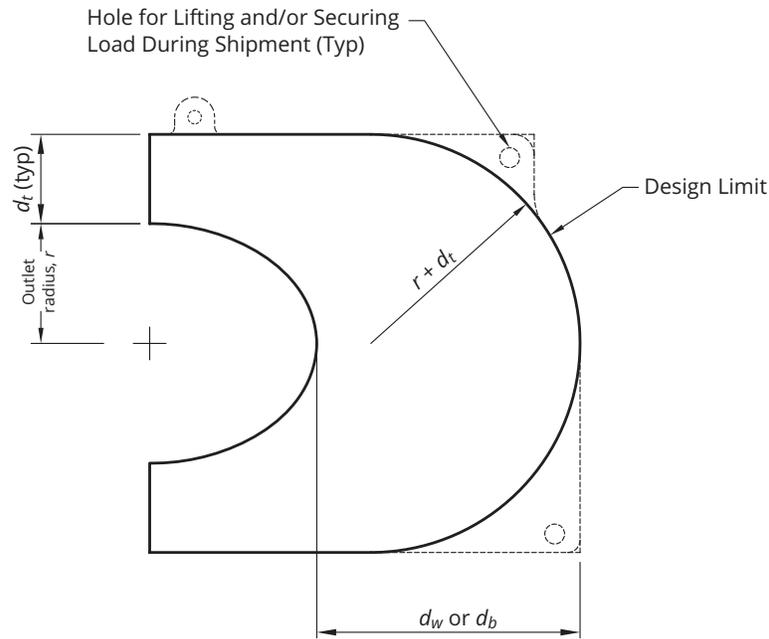
Figure 7-23 Common handling and shipping lifting hole configurations
