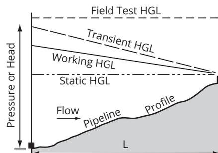
Figure 4-2 Typical pipeline and hydraulic grade profiles for pumped flow
