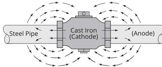
Cast-iron valve is the cathode (protected area), uncoated steel pipe is anode (corroding area), and surrounding earth is the electrolyte. As long as cathode is small in area relative to anode, corrosion is not ordinarily severe or rapid. If these area proportions are reversed, corrosion may be much more rapid.
