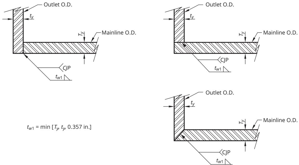
Figure 7-7 Configurations and welding for outlet not requiring reinforcement
