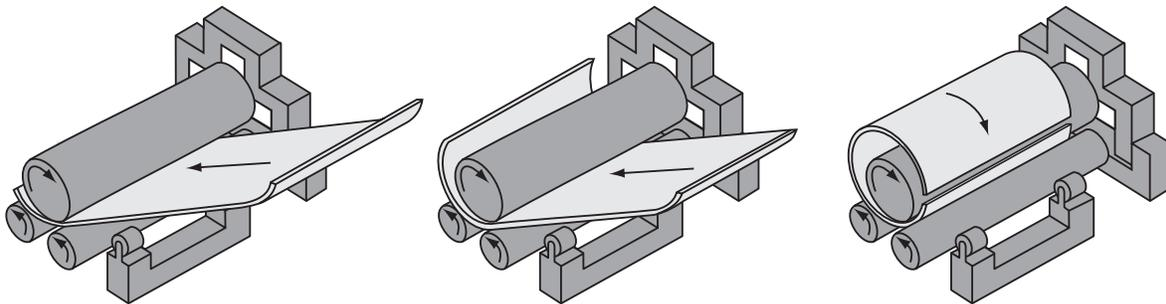
Figure 2-3 Schematic diagram for making plate pipe
